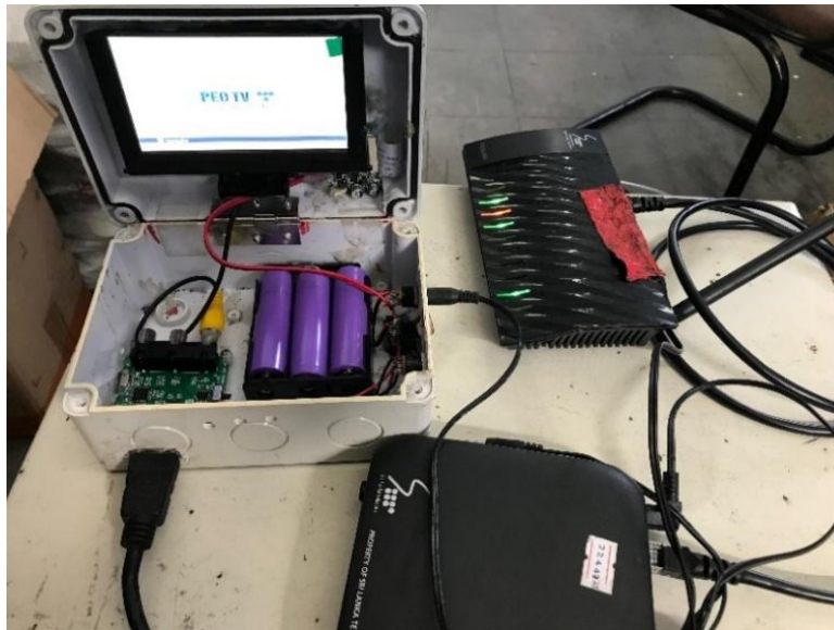
Figure 38: Portable toolkit successfully powering STB, router, and display
