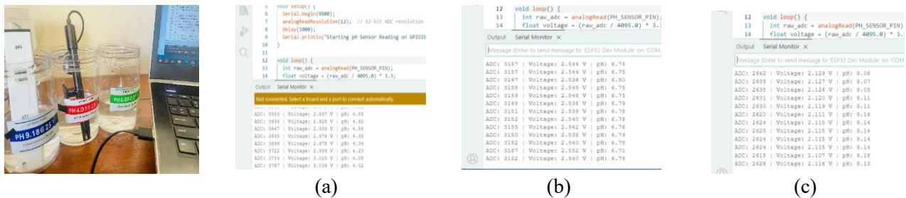
Figure 4: Standard Solutions Used for pH Sensor Calibration (a) 4.01pH solution powder mixed water (b) 6.86pH solution powder mixed water (c) 9.18pH solution powder mixed water
