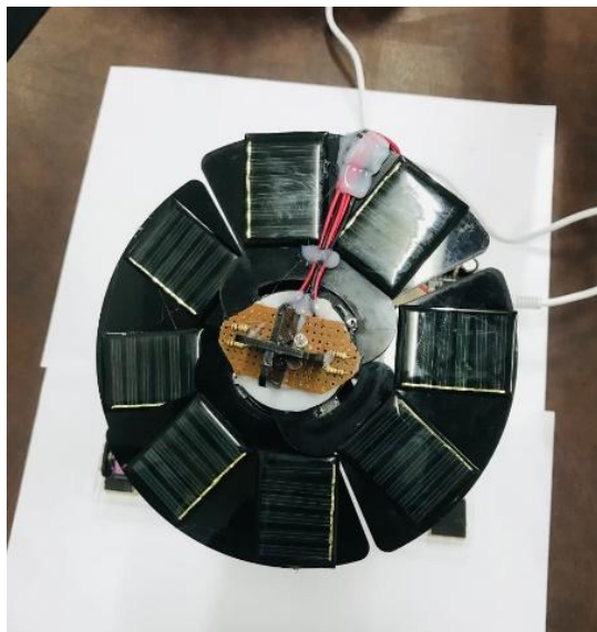
Figure 3.3: Solar tracking system operational tracking position
