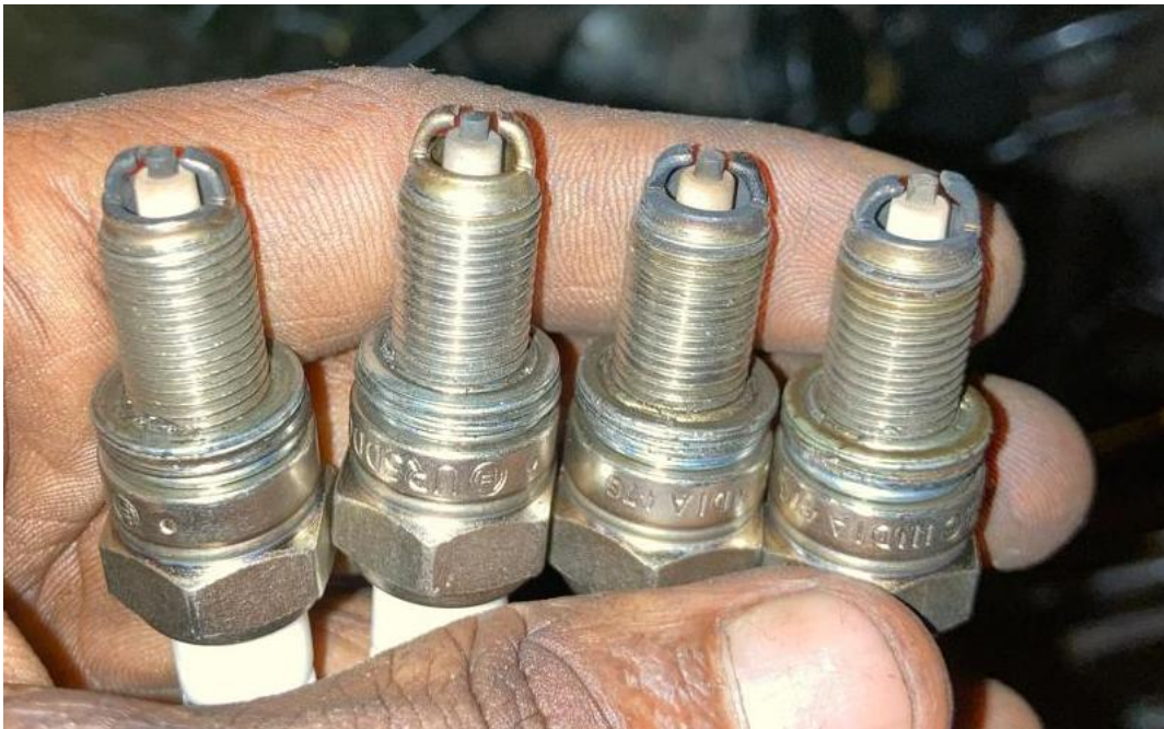
Figure 6: Spark Plugs after test run of the engine
