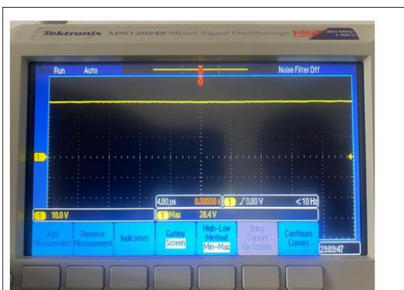
Figure 5: Oscilloscope trace at 28.4 V surge with protection, showing smooth output.
