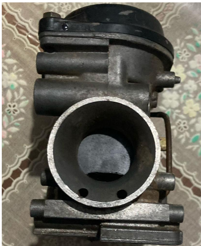
Figure 4: One part of the modified throttle body to correct air flow
