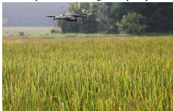
Figure 2.2: Remote sensing drone capturing aerial images for paddy disease detection
