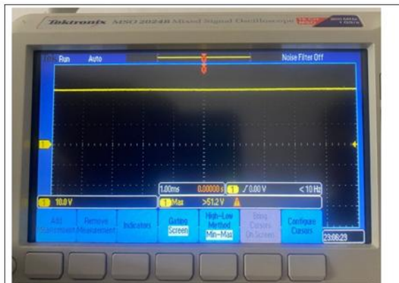
Figure 7: Oscilloscope trace under higher surge with protection, PCB output stable.
