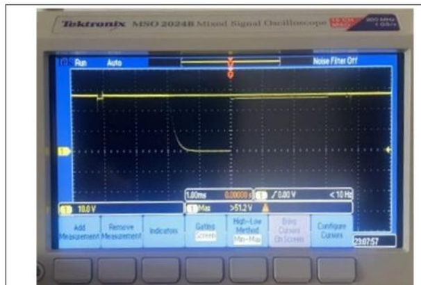
Figure 6: Oscilloscope trace under higher surge without protection, signal unstable.
