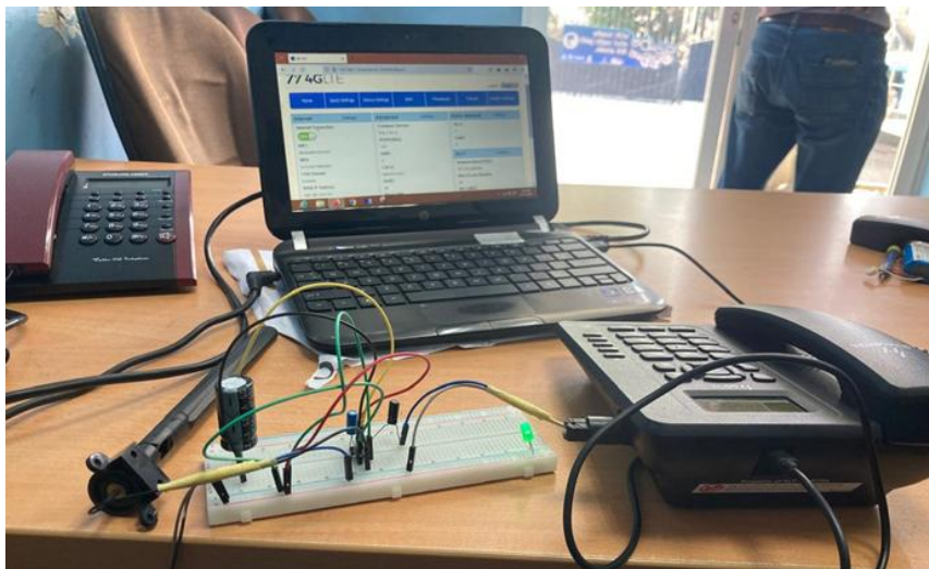
Figure 4: Testing the Signal Booster with LTE Device
