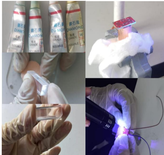
Figure 2.1: Crystal polishing process and SiPM mounting on the NaI(Tl) crystal
