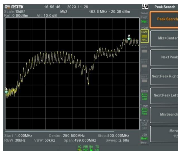
Figure 3.4: Spectrum Analyzer Output after connecting Filter 01 (64 MHz-174 MHz)
