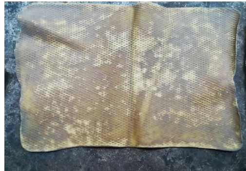
Figure 1.2 Unequally dried rubber sheets
