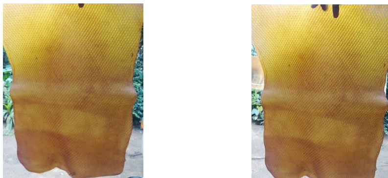
Figure 3.1 Dried Rubber sheet from Solar-powered drying system
