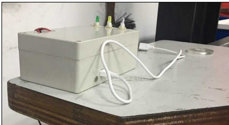
Fig. 5 Control box of the system with LED indicators
