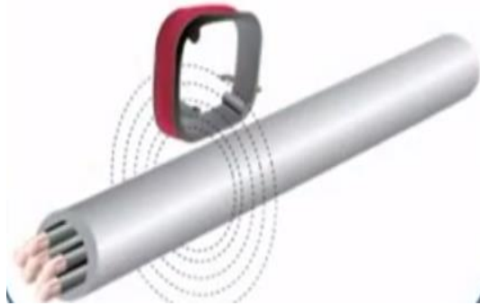
Figure 3: Detecting magnetic flux using the coil
