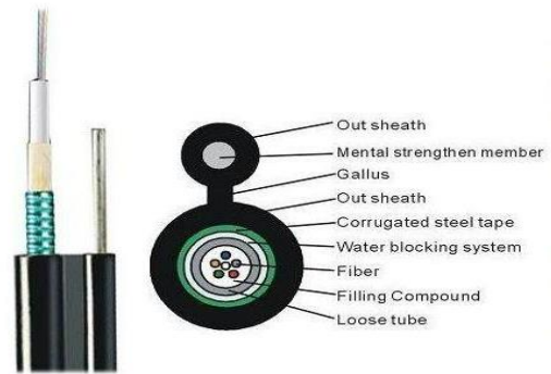
Figure 1: Fiber Cable with Steel Guard wire
