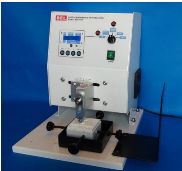
Figure 2: Switch Endurance Test machine
