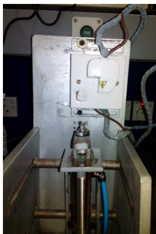
Figure 5: 13A socket test in the tester
