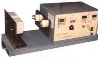
Figure 3: Plug Socket Insertion Endurance Machine
