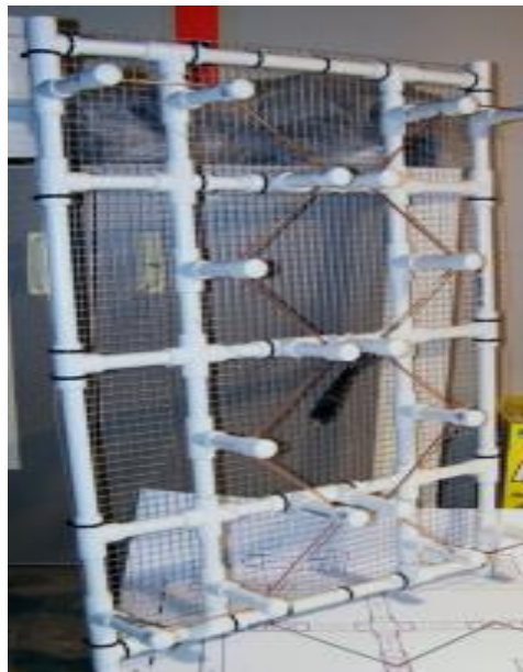
Figure 4: The constructed proposed antenna
