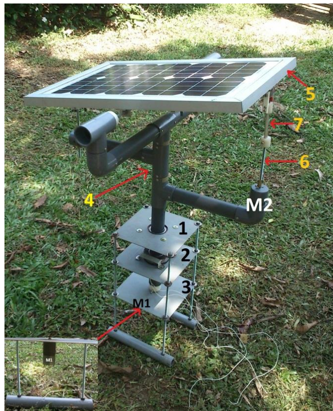
Figure 4: Hardware structure solar tracking system
