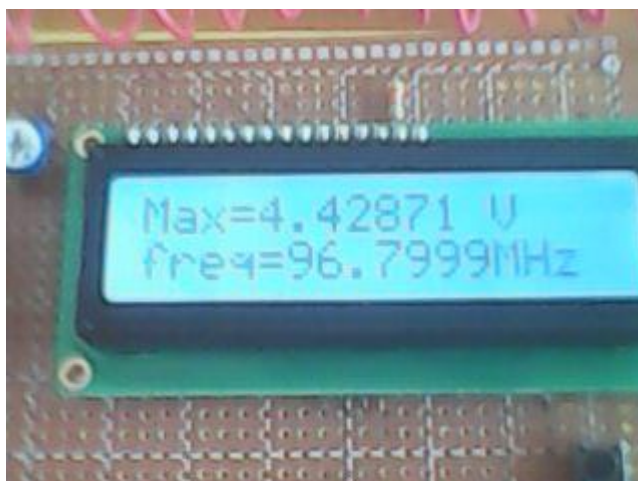
Figure 5: The Result of the one scan cycle is display on the LCD screen
